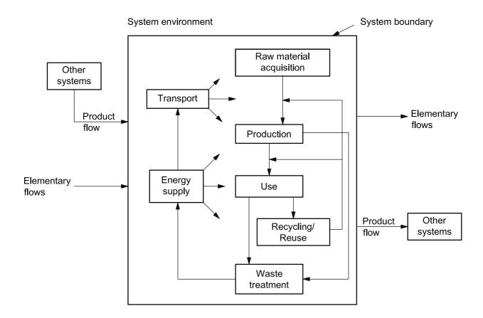
Figure 2 — Example of a product system for LCA
