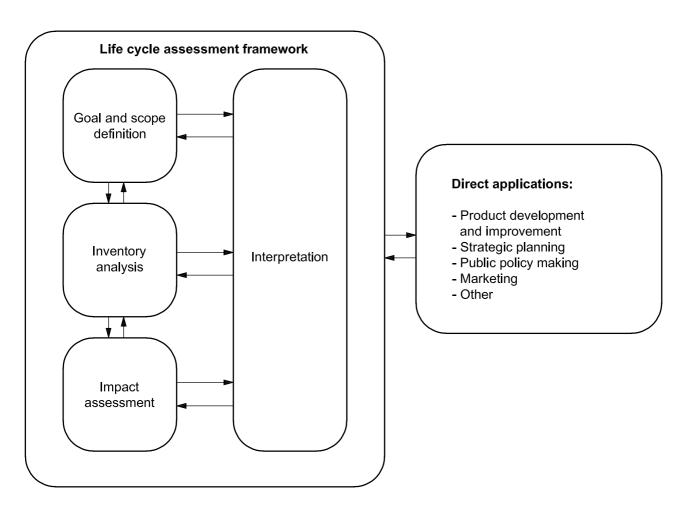
Figure 1 — Stages of an LCA
